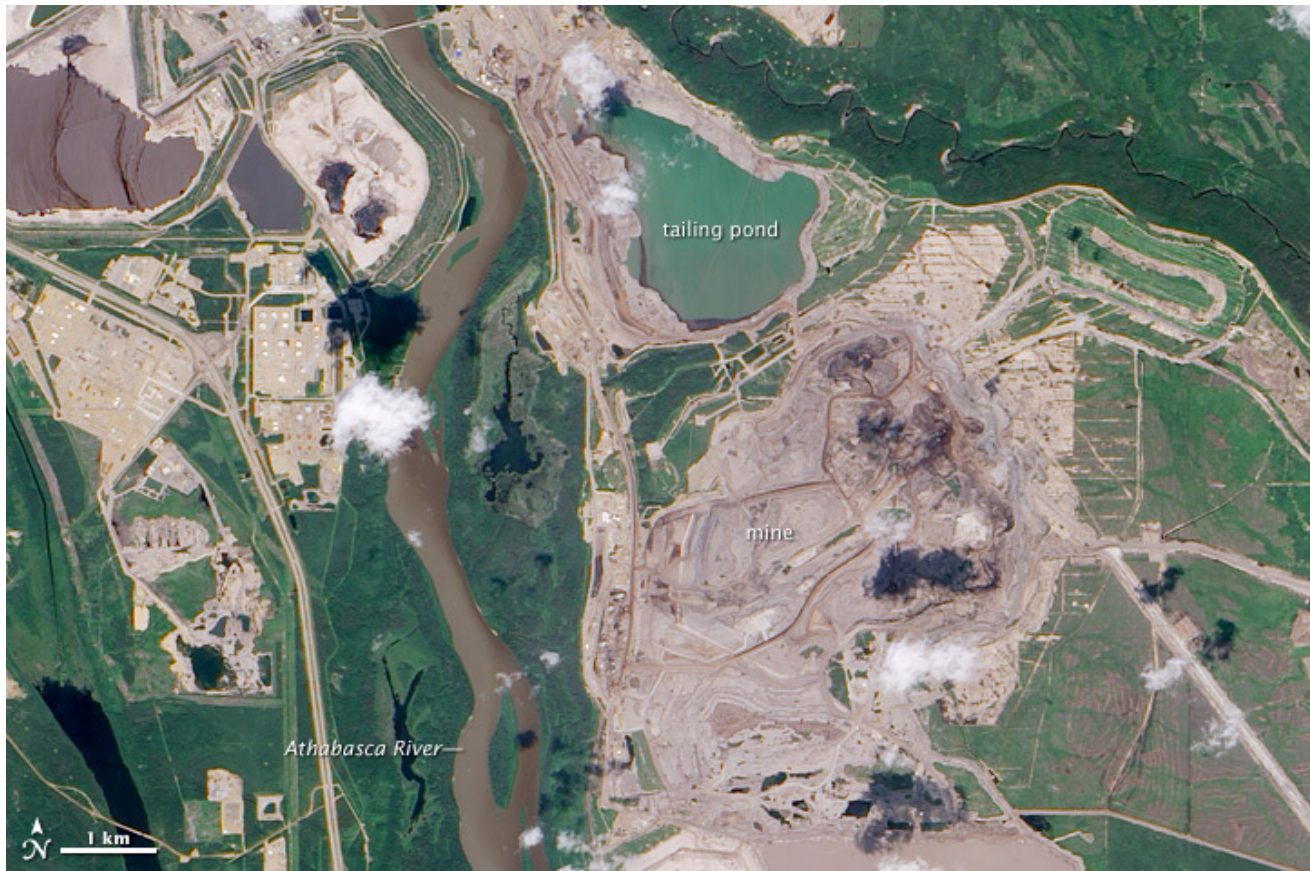
An aerial view of an Athabasca-region oil mine shows the large tailing pond created to hold wastewater. (Photo via NASA )
